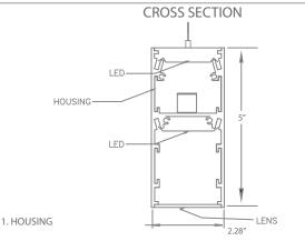
To be formed from 20GA Aluminum Finish: Baked white enamel (standard) Direct / Indirect Lighting (standard) All fixtures are pre-wired All steel parts are phosphate treated for corrosion resistance before painting procedure and then baked with superior adhesion for durability
